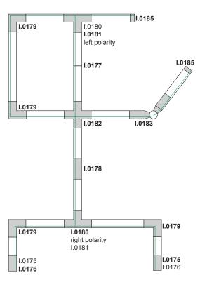
Track is polarized and is manufactured with identifying ridge (green line on diagrams). Refer to these diagrams to ensure proper connector selection.
